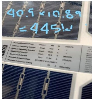
this panel produces 445 watts with a voltage of 40.9 volts and 10.89 amps
